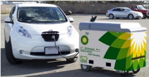
The charger is itself battery-powered of course, and is normally recharged from the mains overnight. It's then capable, during the day, of giving a decent fast-charge to about half a dozen cars (or more, if it can be kept connected to the mains by a suitably long lead for some or all of the day).
